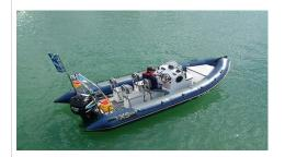
At this sort of size the "serious end" of ribbing will also have double side by side consoles, and multiple seating. What you get in a craft like the XS 600 shown here are typically Deeper V hulls and higher bows than the leisure craft.
