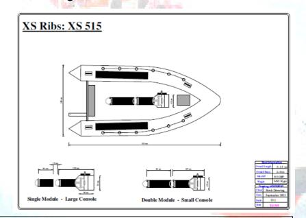
All XS craft are made in the UK, we start with a barrel of resin and a roll of fabric and make the whole boat IN HOUSE at our factory in Yorkshire. All metal work, fuel tanks, steering and fittings are sourced in the UK and are supplied to the relevant ISO standard for the item. All consoles and seating are BONDED to the deck, NOT screwed down. We pride ourselves in the quality we deliver. This is why these craft do the job and last, durability is BUILT IN.
