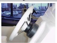
referred to for maintenance and service instructions. **LEFT:** Hydraulic steering, note filler cap for fluid on top of unit. Hydraulic steering MAY OR MAY NOT be a tilting unit. (Tilting unit shown) **RIGHT:** Mechanical steering
