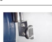
Use the two transom U bolts fitted to the outside of the transom to tow other craft or water sports activities, they are strong points suitable for towing from. There exact position will vary from craft to craft and they MAY be used to secure the A frame on.
