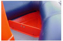
primarily to prevent rope sliding back in the boat. Use the eye bolt on the inside of the external bow eye to bear any load, the cleat and eye bolt on the wall are for securing the rope ends to.
