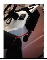
**SAFETY LANYARD::** this MUST be worn at all times when the motor is running, if the throttle is inadvertently operated when the boat is at rest the consequences of being unable to stop the craft can be very serious. The Lanyard must securely fixed to the driver, do not use loops on clothing or zip toggles that can break under load, clip the safety lanyard back to its self.
