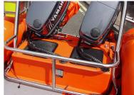
A stern locker is an option, this is used to house battery(s) and oil tanks. The exit to the under deck loom if fitted will be inside this locker. Care should be taken when trimming engine up to avoid trapping anything on top of the locker as this may damage the engine control wires and cables.
