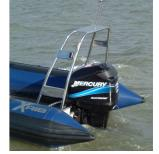
Stability of the craft may be affected if heavy objects are carried on the frame, the frame is NOT designed to carry heavy objects.
