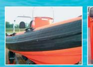
Triple Rubber Strake: Two Fire extra flat sections of strake above Extinguisher Steel A-Frame and below the main D-section. in recess -The cleat style rubber handle is fitted into also visible in this picture. seat unit.
