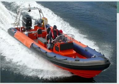
The XS 850 has the payload capacity to carry substantial loads as well as have an immense range if the largest fuel tank options are fitted. This craft needs a minimum of a single 225 hp outboard and is well suited to twin outboards of upto 250 hp. It will also suit single and some twin diesel inboard installations.
